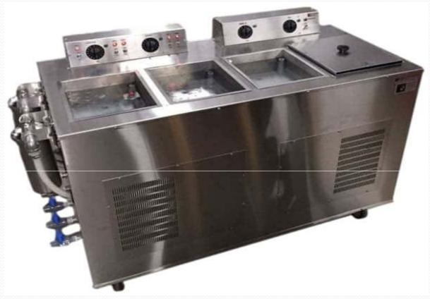
Spray Cleaning, Ultrasonic Cleaning, Rinsing & Drying stations as per requirement Available in manual transfer & Auto transfer Features : Heater with Temperature Controller Filtration & Recycling Oil Skimmer PLC logic operations HMI for Set Value & Process Value
