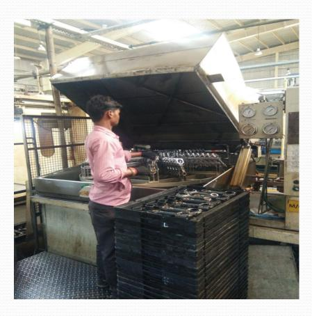
Suitable for components to qualify Millipore value Features : Heater with Temperature Controller Filtration & Recycling Oil Skimmer PLC logic operations HMI for Set Value & Process Value
