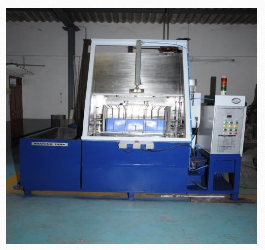
Two Stage – Soaking & Pressure Cleaning Suitable for Heavy muck removal
