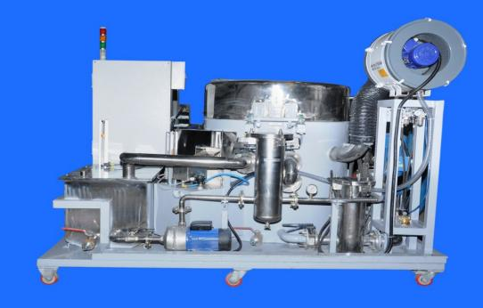
Features : Heater with Temperature Controller Filtration & Recycling Oil Skimmer PLC logic operations HMI for Set Value & Process Value
